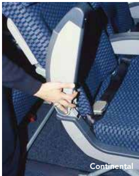
Above: The armrests of some aisle-side seats can be raised to help passengers with disabilities gain access to their seat rows more easily.
