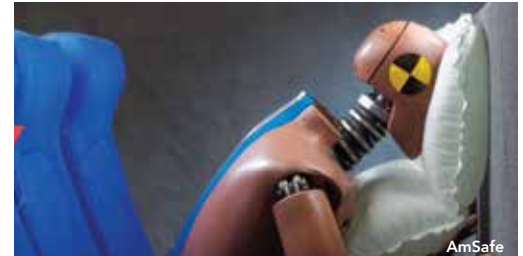
Left: An airbag is contained within the belt, alongside the buckle.
