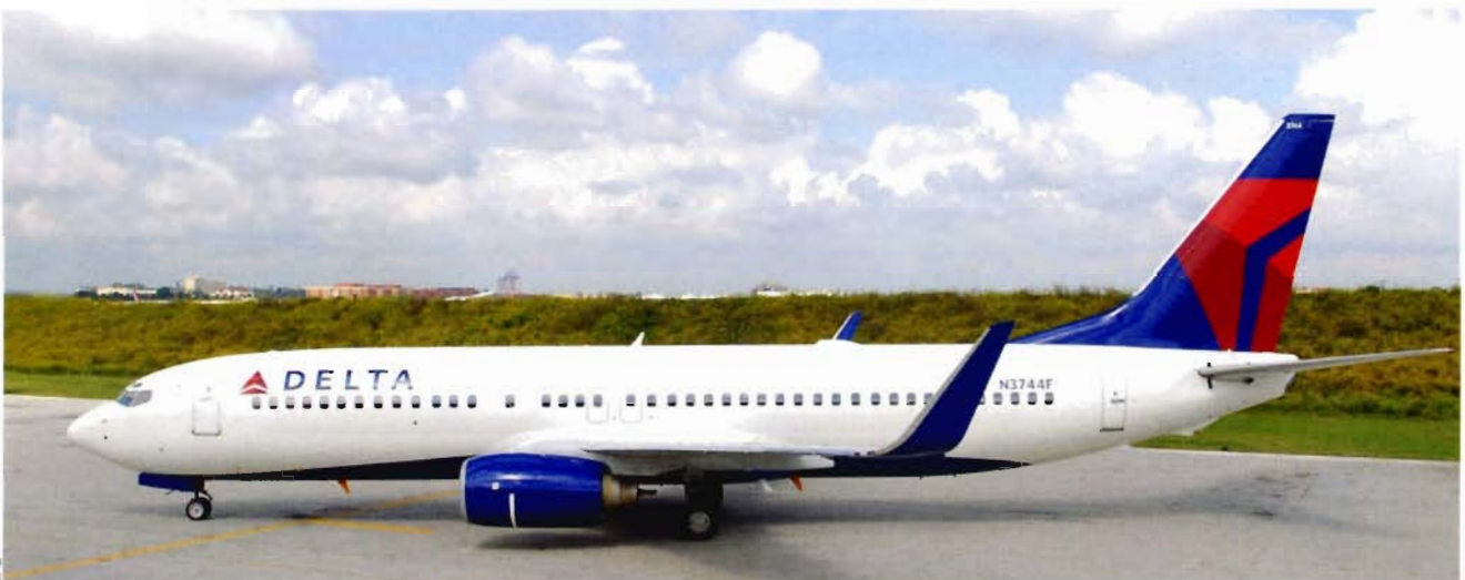
Aviation Partners Boeing blended winglets are being fitted to 737-800s (pictured), 757s, and 767s.
